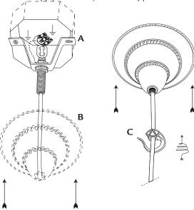
5. Screw the hook **C** onto the nipple and tighten securely.
