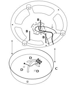
5. Secure the cover against the fixture **A** screwing the 3 screws E on the 3 nipples **B**.
