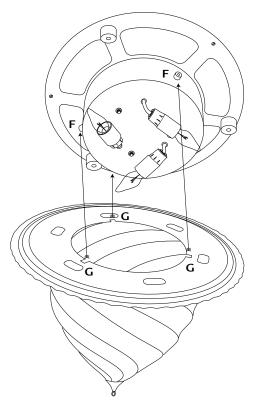
8. Suspend the drop. Restore the electricity and test.
