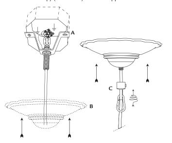
5. Screw the hook **C** onto the nipple and tighten securely.
