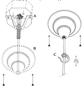
5. Screw the hook **C** onto the nipple and tighten securely.
