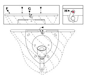
7. Install bulb. Do not exceed the maximum wattage for this fixture. Refer to the wattage warning label attached to the fixture for maximum allowable wattage.
