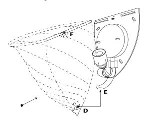
To secure the fixture against the mounting surface hang the element F to the mounting bracket as shown. Turn the hook G and fix it using the screw H.
