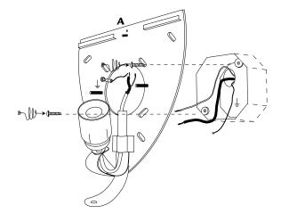
Place the metal plate B over element A so that the threaded studs extends through the 2 holes. Secure against the mounting surface using the 2 mounting caps C provided.
